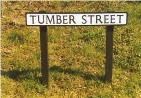
7 Highlight local names and features of historic interest. For street names, traditional looking black and white signs are generally preferable. Recycled plastic posts (as shown) are acceptable for most situations.
